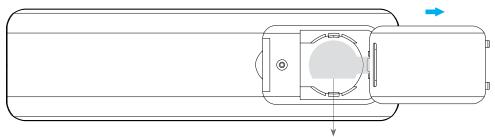
Note: before the first use, please remove the protective film on the battery.
